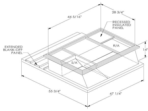
ONE PIECE WELDED CONSTRUCTION
