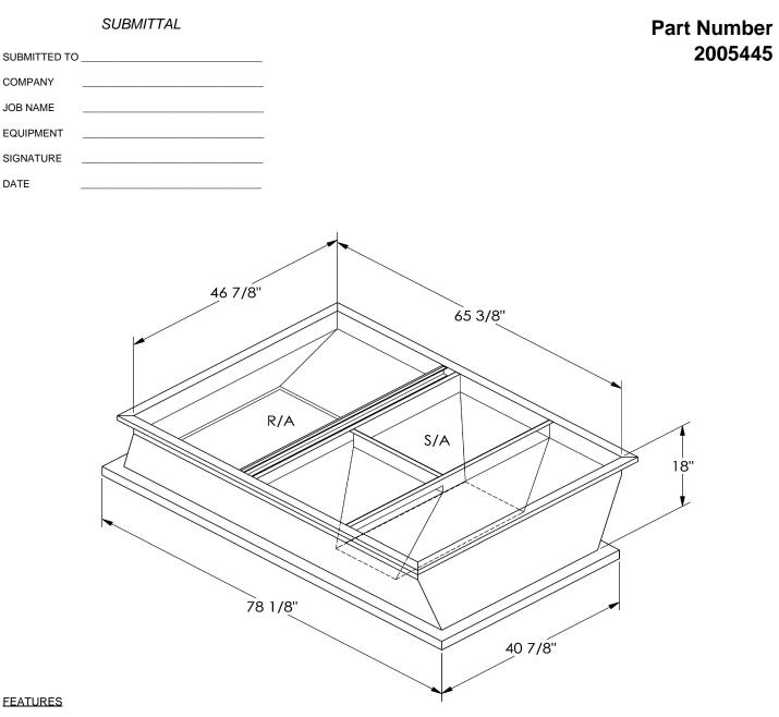
ONE PIECE WELDED CONSTRUCTION
