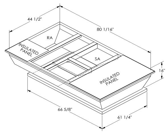
ONE PIECE WELDED CONSTRUCTION
