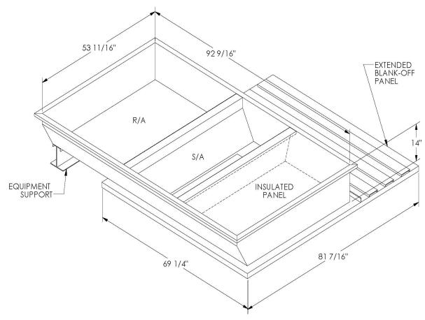
ONE PIECE WELDED CONSTRUCTION
