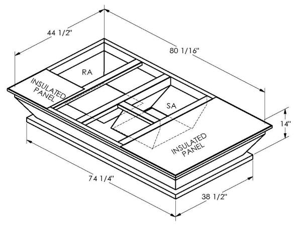
ONE PIECE WELDED CONSTRUCTION
