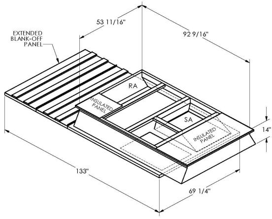
ONE PIECE WELDED CONSTRUCTION
