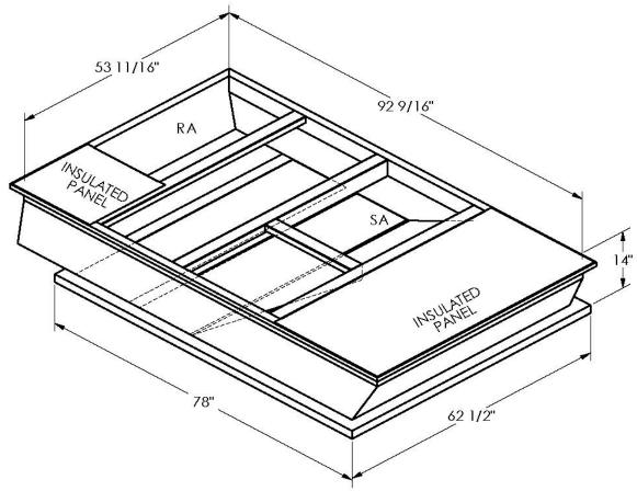
ONE PIECE WELDED CONSTRUCTION
