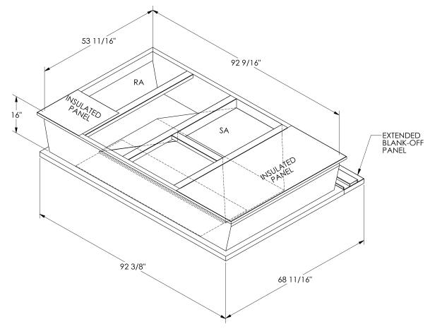
ONE PIECE WELDED CONSTRUCTION
