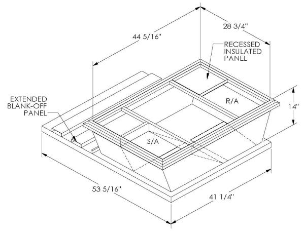
ONE PIECE WELDED CONSTRUCTION
