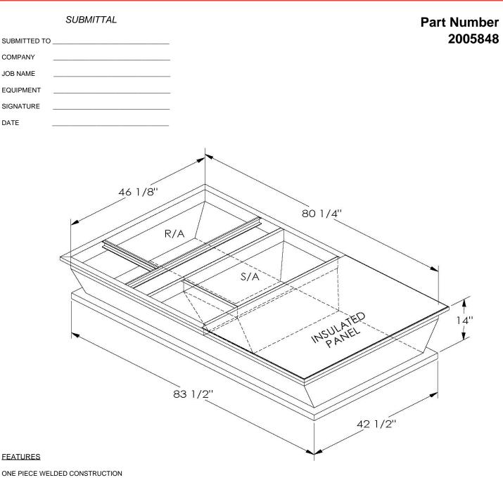
FACTORY INSTALLED SUPPLY TRANSITIONS
