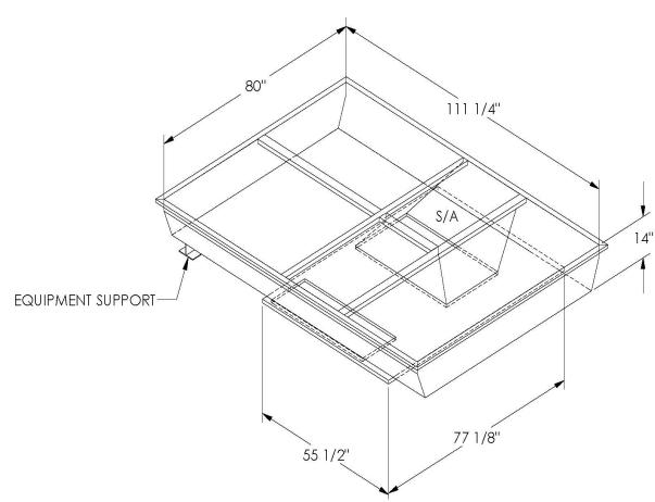
ONE PIECE WELDED CONSTRUCTION
