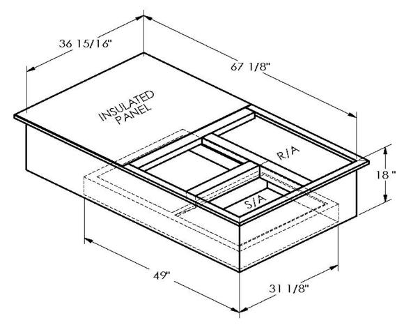
ONE PIECE WELDED CONSTRUCTION
