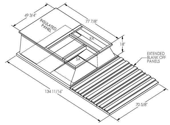
ONE PIECE WELDED CONSTRUCTION
