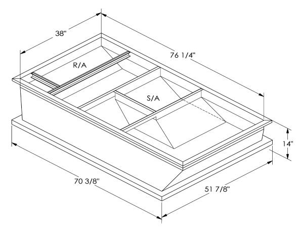
ONE PIECE WELDED CONSTRUCTION
