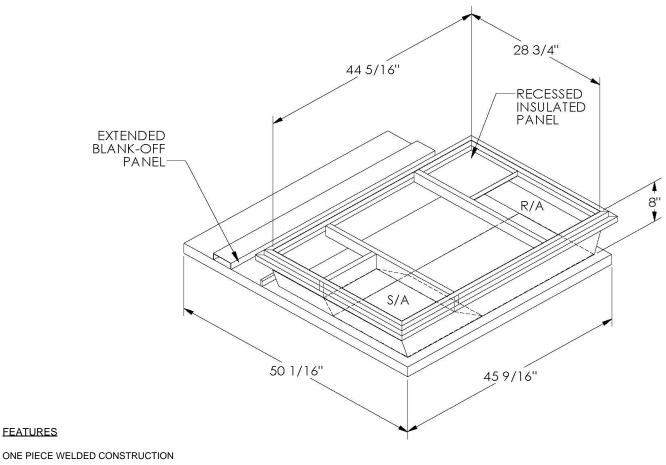
FACTORY INSTALLED SUPPLY TRANSITIONS
