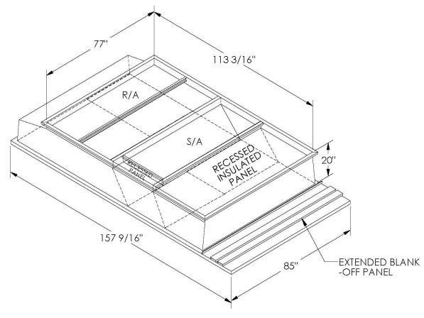
ONE PIECE WELDED CONSTRUCTION
