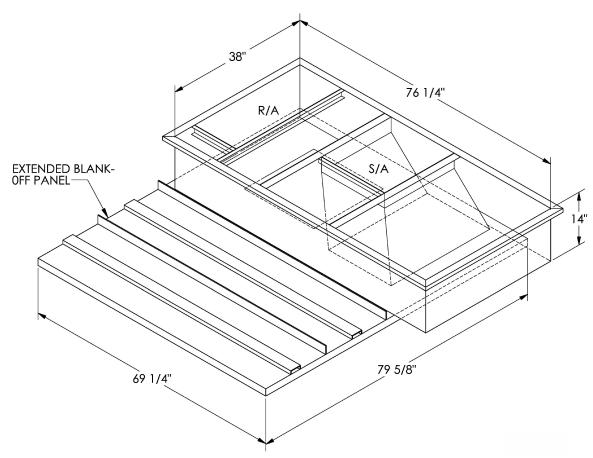
ONE PIECE WELDED CONSTRUCTION
