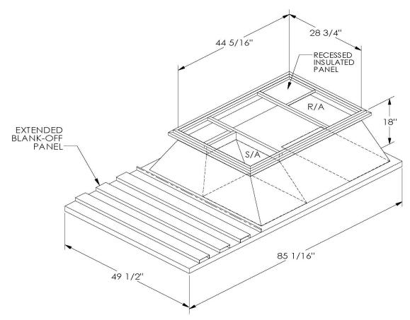
ONE PIECE WELDED CONSTRUCTION
