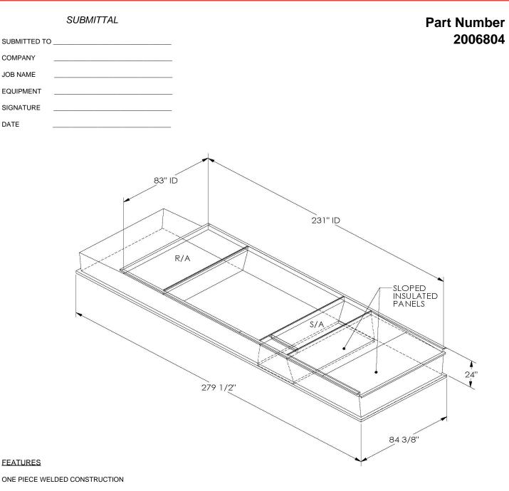
FACTORY INSTALLED SUPPLY TRANSITIONS
