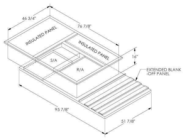
ONE PIECE WELDED CONSTRUCTION
