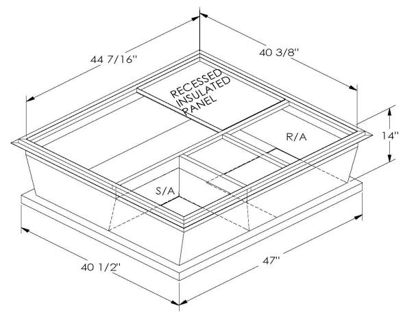
ONE PIECE WELDED CONSTRUCTION
