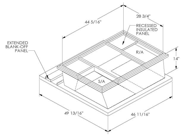
ONE PIECE WELDED CONSTRUCTION
