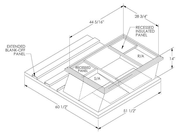
ONE PIECE WELDED CONSTRUCTION
