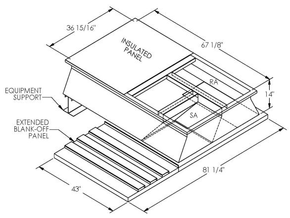
ONE PIECE WELDED CONSTRUCTION
