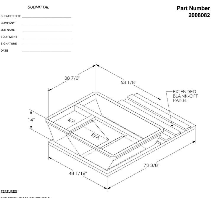
ONE PIECE WELDED CONSTRUCTION
