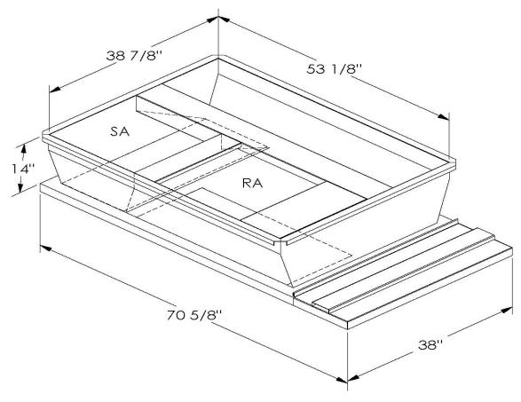
ONE PIECE WELDED CONSTRUCTION
