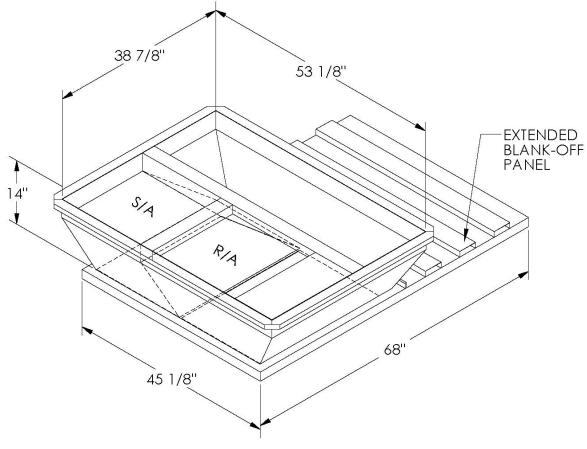
ONE PIECE WELDED CONSTRUCTION
