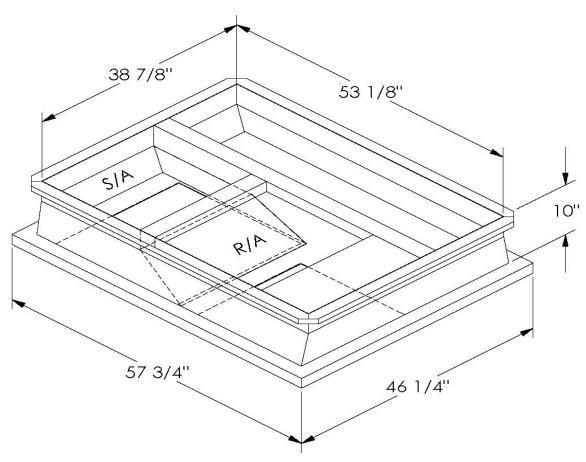
ONE PIECE WELDED CONSTRUCTION
