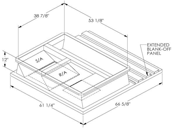
ONE PIECE WELDED CONSTRUCTION
