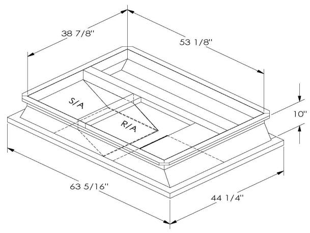
ONE PIECE WELDED CONSTRUCTION
