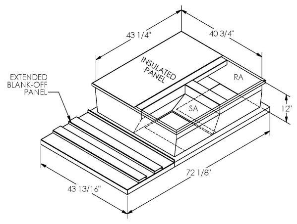
ONE PIECE WELDED CONSTRUCTION
