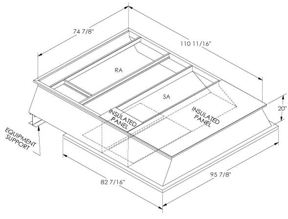
ONE PIECE WELDED CONSTRUCTION
