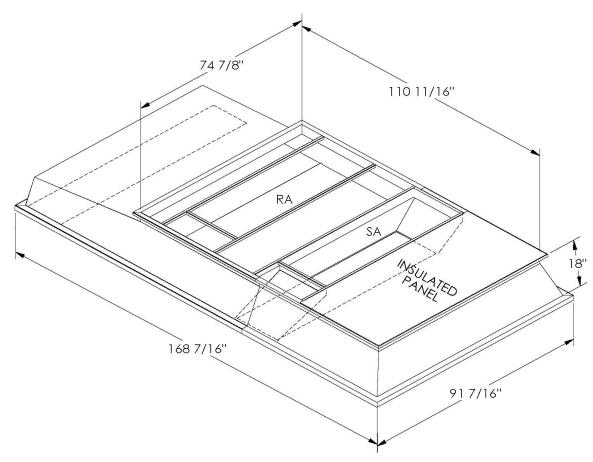
ONE PIECE WELDED CONSTRUCTION
