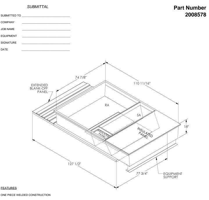
FACTORY INSTALLED SUPPLY TRANSITIONS
