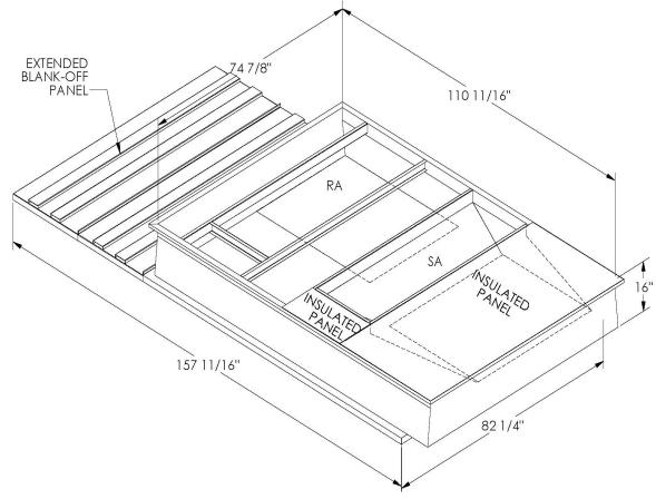
ONE PIECE WELDED CONSTRUCTION
