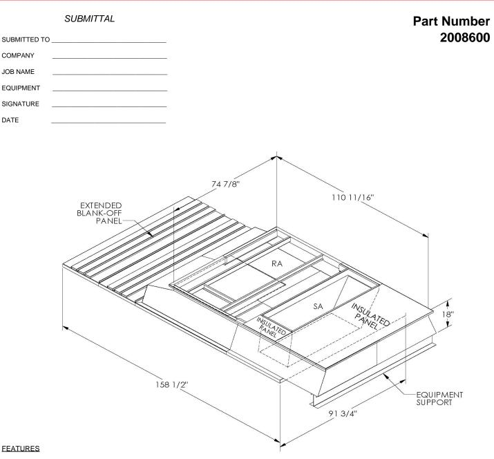
ONE PIECE WELDED CONSTRUCTION
