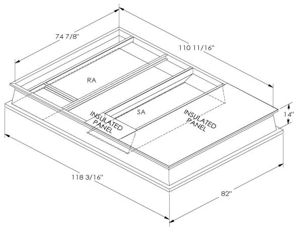
ONE PIECE WELDED CONSTRUCTION
