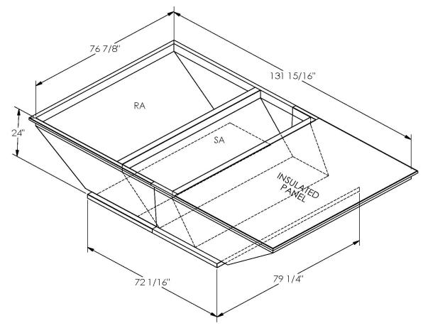
ONE PIECE WELDED CONSTRUCTION
