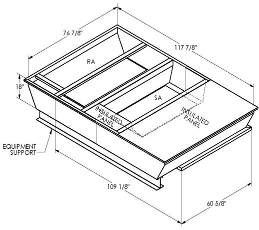
ONE PIECE WELDED CONSTRUCTION
