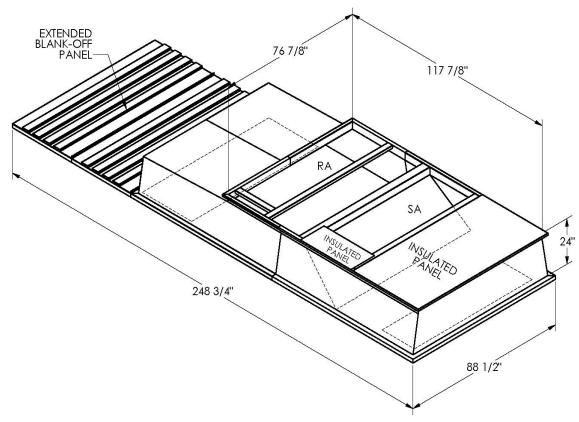
ONE PIECE WELDED CONSTRUCTION
