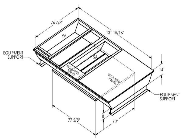
ONE PIECE WELDED CONSTRUCTION
