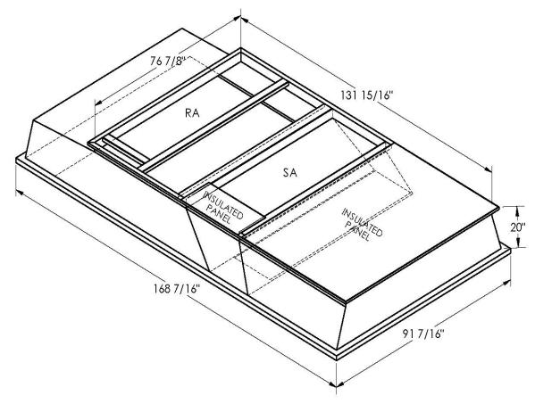
ONE PIECE WELDED CONSTRUCTION
