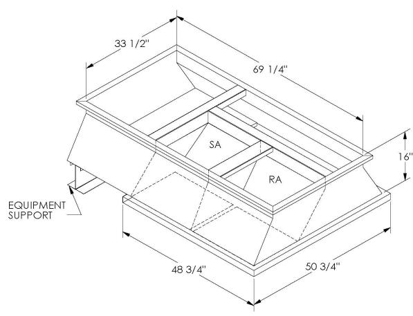
ONE PIECE WELDED CONSTRUCTION
