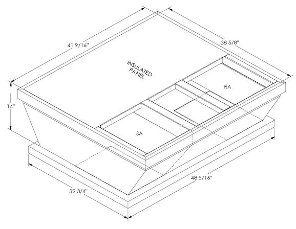
ONE PIECE WELDED CONSTRUCTION
