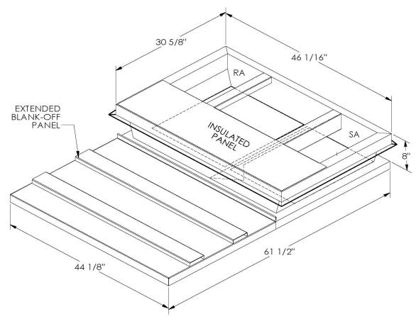
ONE PIECE WELDED CONSTRUCTION
