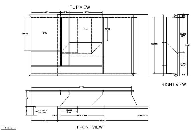
ONE PIECE WELDED CONSTRUCTION
