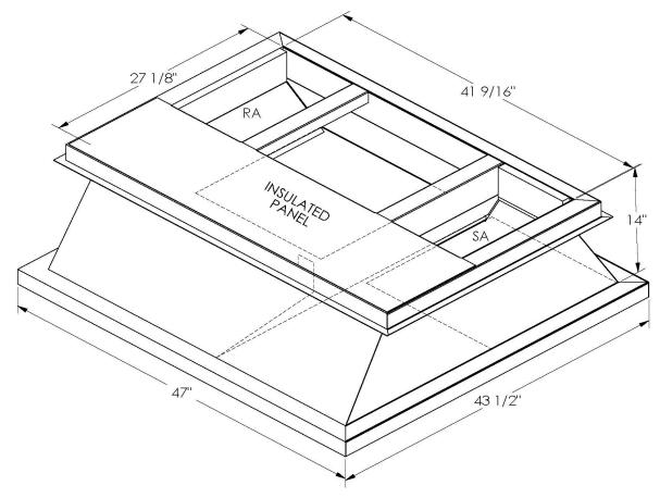
ONE PIECE WELDED CONSTRUCTION
