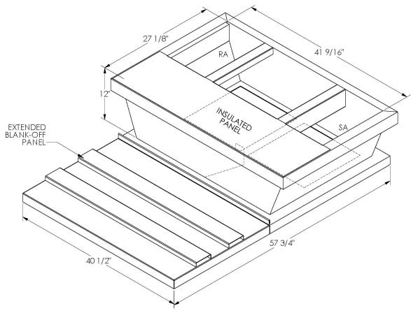
ONE PIECE WELDED CONSTRUCTION
