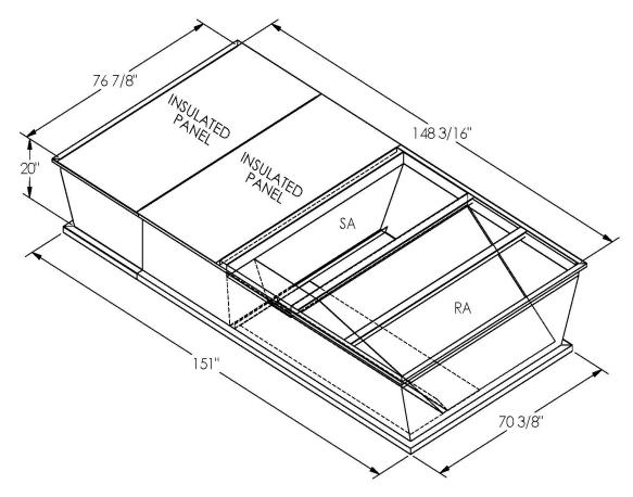
ONE PIECE WELDED CONSTRUCTION
