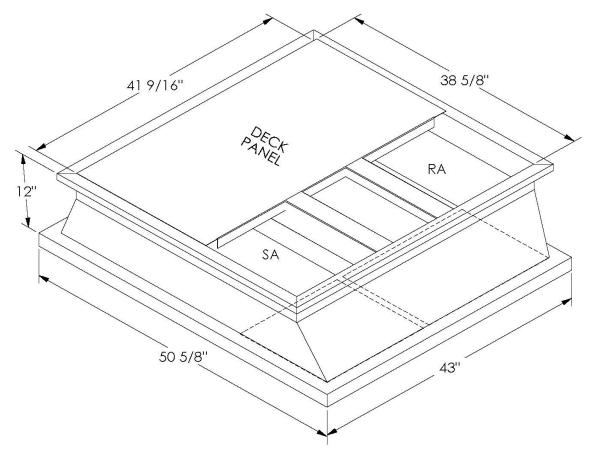
ONE PIECE WELDED CONSTRUCTION
